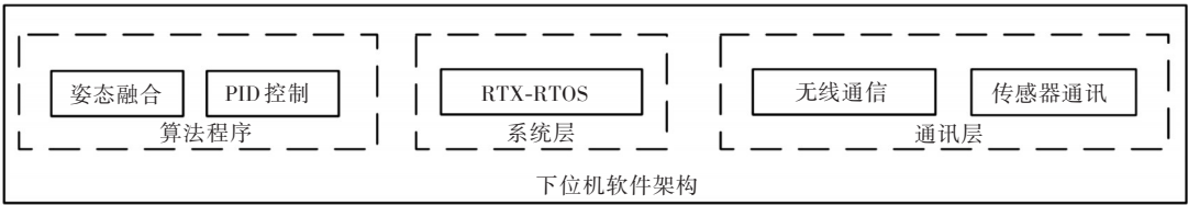
图9 下位机软件架构图 Fig. 9 Software architecture diagram of lower computer
