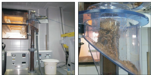
Fig. 3 Column flotation (3 inches diameter) applied to the apatite rougher flotation tests
