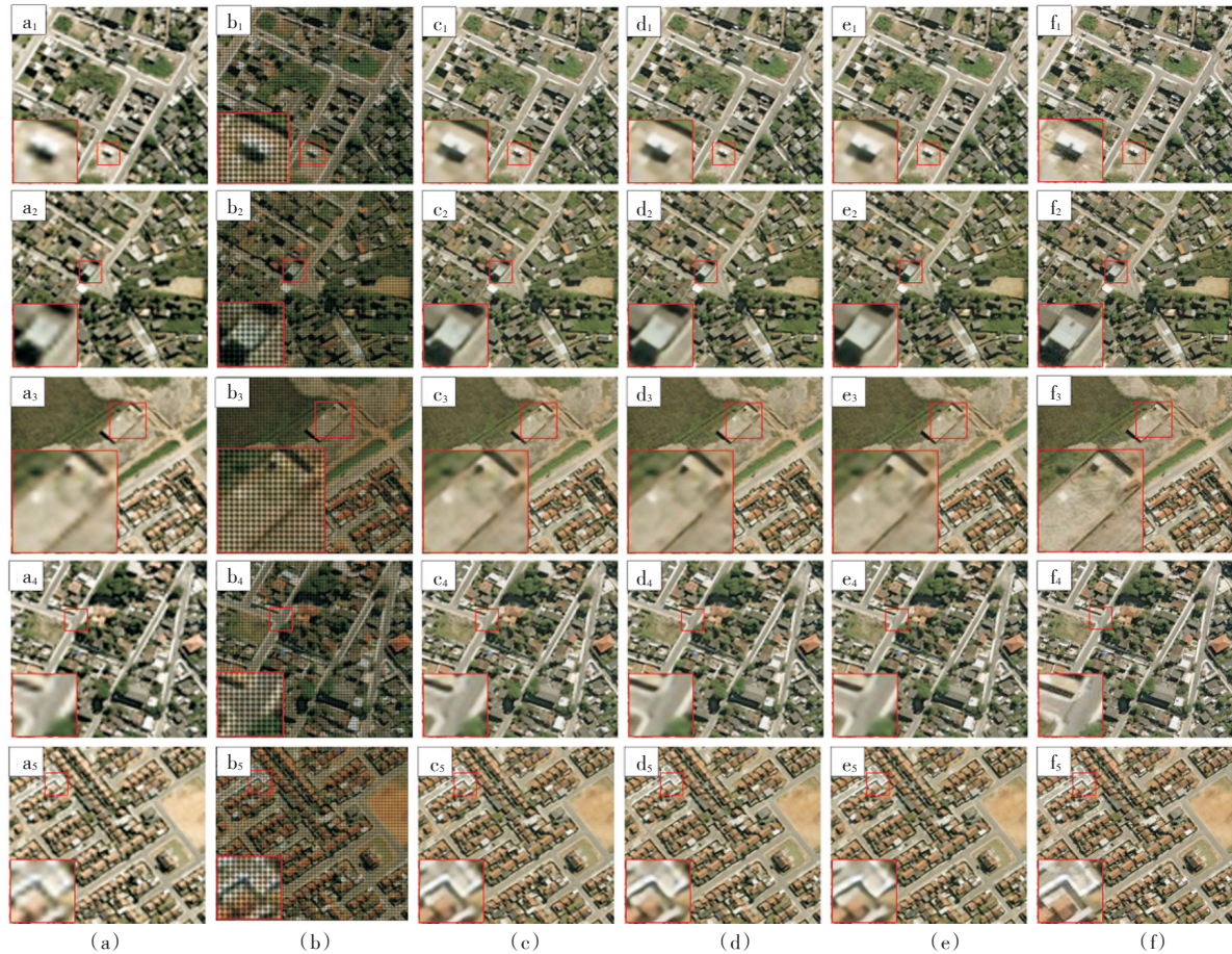
图4 SpaceNet卫星图像超分辨率结果的主观对比: (a)双三次插值, (b)FSRCNN, (c)LapSRN, (d)VISR, (e)本文算法, (f)高分辨图像
